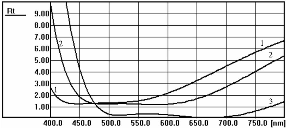
Fig. 6. Reflectance diopter 1, uniform optical coating: 1 – non-optimized; 2- optimized; 3 – optical coating , normal incidence
