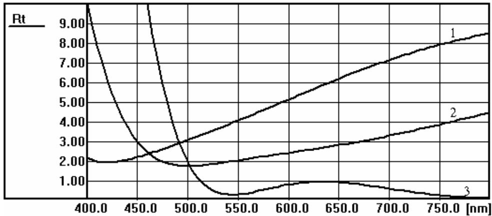
Fig. 7. Reflectance diopter 1, non-uniform optical coating : 1 – non-optimized; 2- optimized; 3 – optical coating , normal incidence
