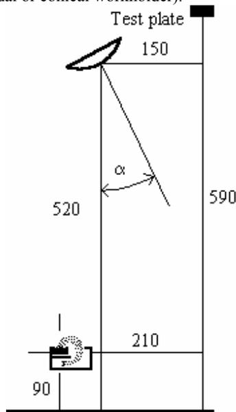
Fig. 3 The geometry of evaporation. Dimensions are in mm.
