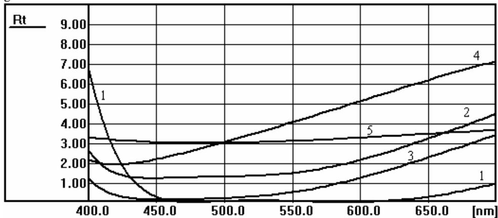
Fig. 5. Reflectance diopter 1. 1-normal incidence; 2 – uniform coating, aperture  $40^\circ$ ;
